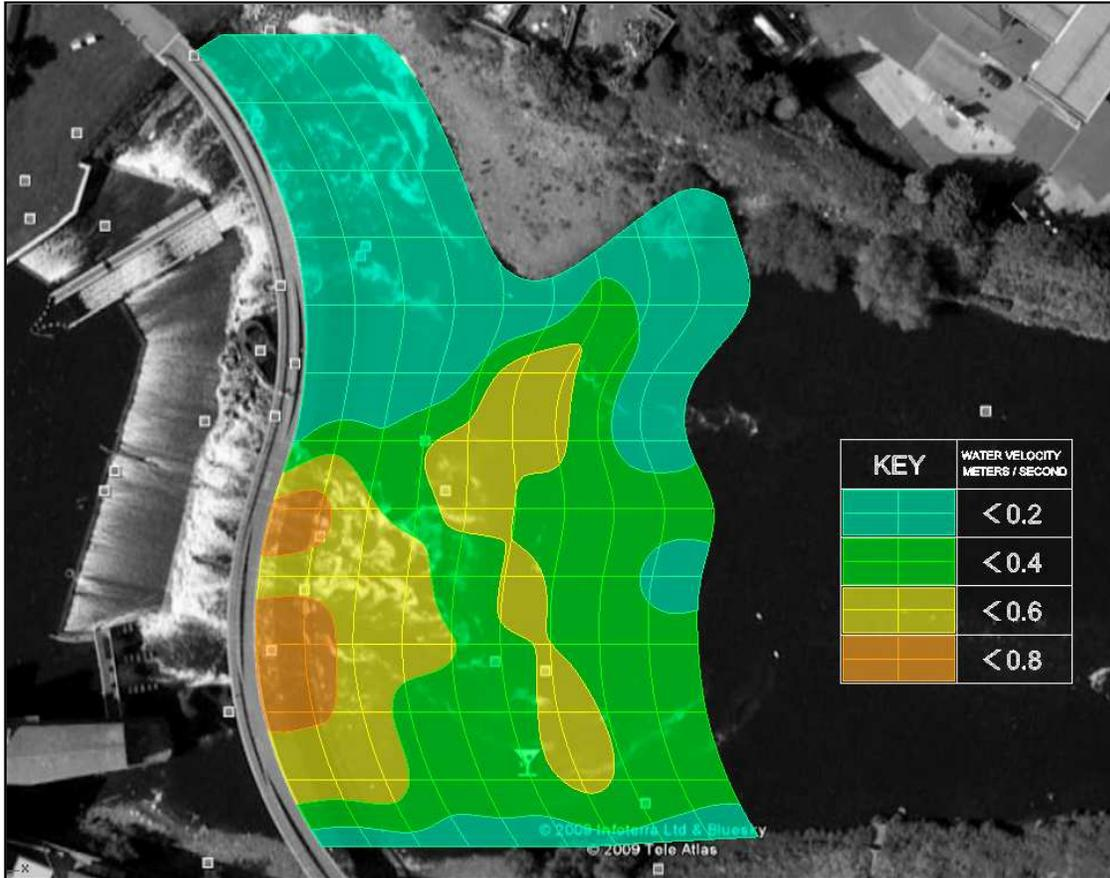
**Figure 10: predicted alterations to water velocities in Castleford Mill weir pool, based on the flows already reported and a turbine abstraction of 30 cumecs**
