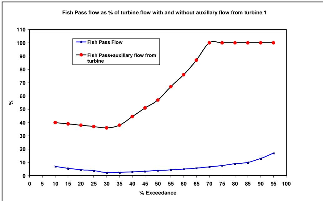
Figure 13: fish pass attraction flow as a % of turbine flow
