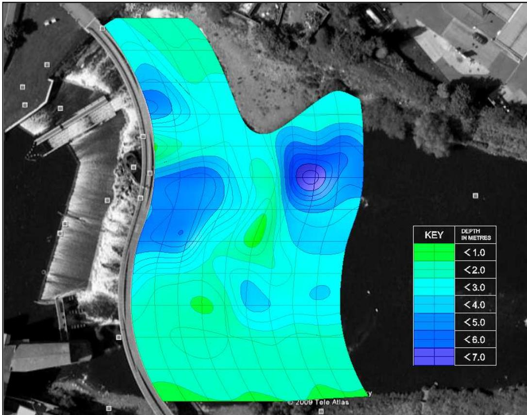
**Figure 8: schematic map illustrating the depths throughout Castleford Mill weir pool**
