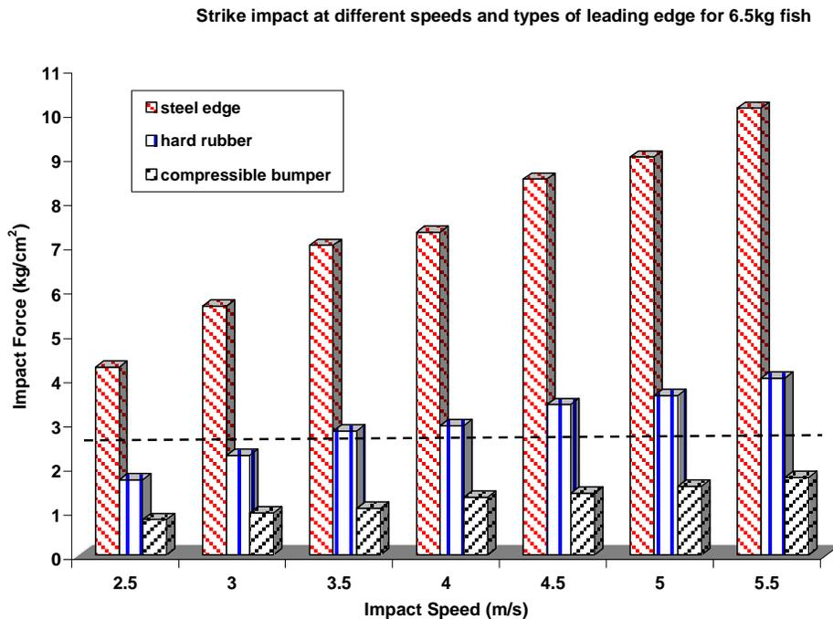
**Figure 7: the strike impact force exerted by different leading edge types on a 6.5 kg fish**
