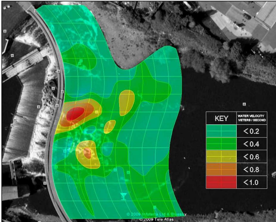
**Figure 9: schematic map illustrating the water velocities throughout Castleford Mill weir pool**
