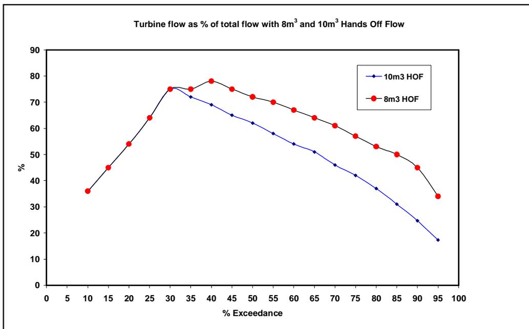
Figure 14: attraction flow from the turbines as % of total flow with different HOFs
