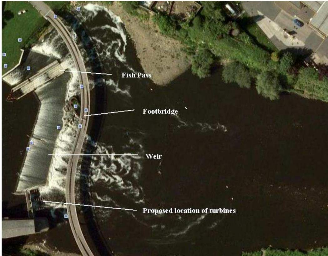
Figure 1b: aerial photograph of the weir pool at Castleford. The location of the proposed turbine installation is given
