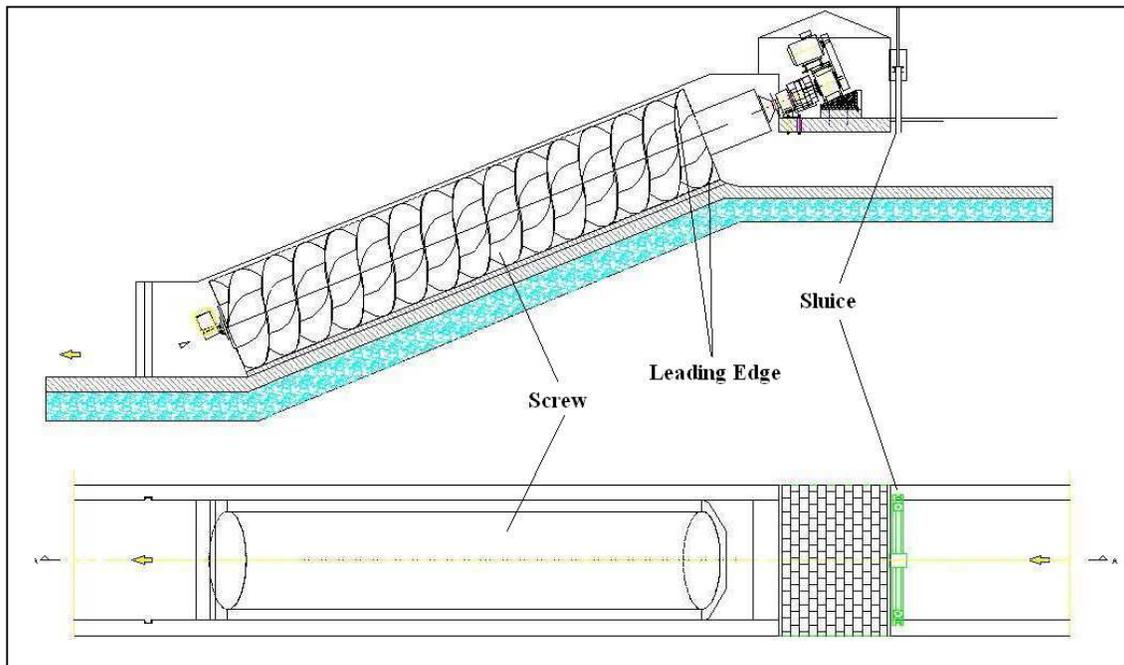
**Figure 2: Diagram of an Archimedes hydraulic turbine, shown from the side (top) and overhead (bottom)**
